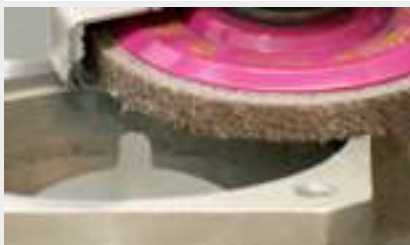
Aluminium: for cleaning and fine grinding
